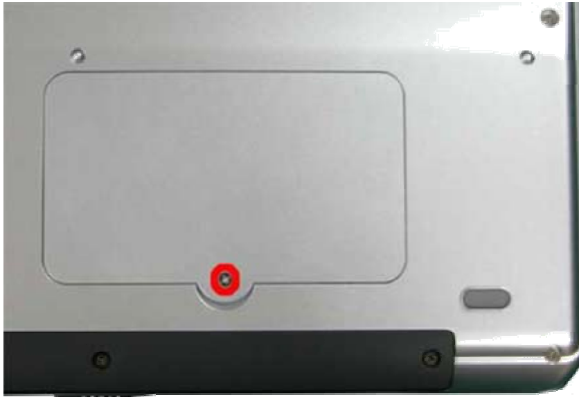
Fig. 2 Removing the screw retaining the memory module slot cover
